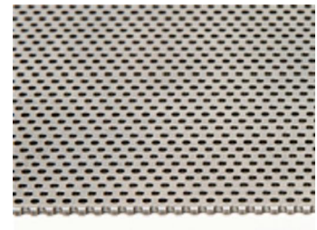
SUS304L (Open Area 22.6%) t2×D1.5×P3 60deg. Staggered
