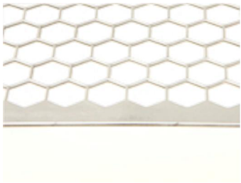
SUS304 t1.5×Regular Hexagon12× P13 60deg. Staggered
